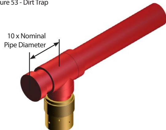
Figure 53 - Dirt Trap
