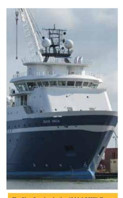
The Blue Orca has both a Kidde<sup>®</sup> ECS<sup>™</sup> Clean Agent System with 3M<sup>™</sup> Novec<sup>™</sup> 1230 Fluid and a Kidde High-Pressure Carbon Dioxide System installed onboard. Our systems are protecting the Engine Room and Casing, Emergency Generator, Brake Frac Pump, Sand Silo and Generator Rooms.
